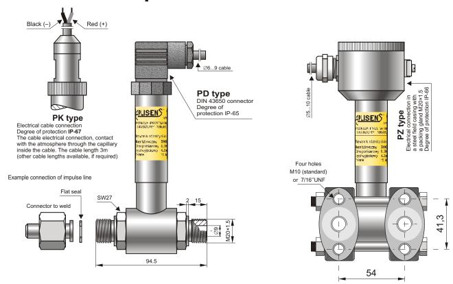
**Transmitter PRE-28**Process connection **P type**Static pressure limit 40 bar
