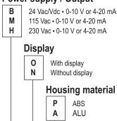
$\begin{tabular}{ll} \textbf{Example: CP302-BOA} = pressure transmitter type CP 300, with measuring range of $-500/+500$ Pa, with power supply $24$ Vac/Vdc, 0-10 V or 4-20 mA output, $-200/+200 mA outpu$ with display and alu housing.
