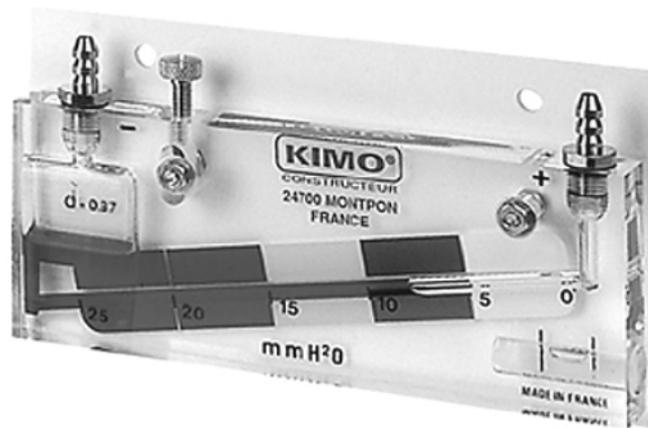
The CP 25 inclined liquid column manometer, developed and manufactured by KIMO measures slight variations in pressure, depression or differential pressure of air or gas. It is specially designed for checking clogging of filters in painting booths.
