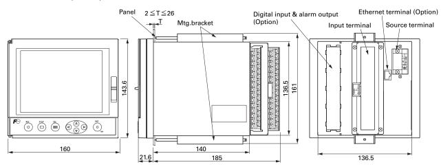
(Note) When placing the main unit on another instrument or on the floor, allow a space of 100mm or more between the unit and instrument or the floor.
