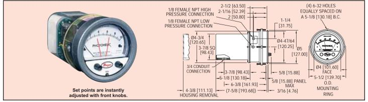
Photohelic® Switch/Gages function as versatile, highly repeatable pressure switches combined with a precise pressure gage employing the time-proven Magnehelic® gage design. The Photohelic® gage measures and controls positive, negative or differential pressures of air and compatible gases. Standard models are rated to 25 psig (1.7 bar) with options to 35 (2.4) or 80 (5.5 bar) psig. Single pressure 36000S models measure to 6000 psig (413 bar) with a 9000 psig (620 bar) rating.
