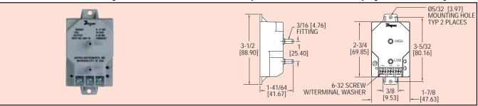
Our low cost Series 668 Differential Pressure Transmitter is capable of measuring low pressures with a  $\pm 1\%$  accuracy — ideally suited for proper building pressurization and air flow control. Transmitters can withstand up to 10 psig overpressure with no damage to the unit. Variable capacitance sensor design provides excellent sensitivity and long-term stability. Compact, lightweight design makes installation simple and easy. Units also feature reverse-polarity protection.
