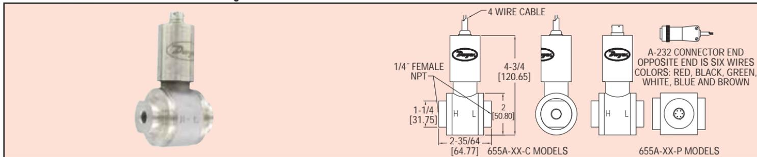
**Series 655A Differential Pressure Transmitters** are designed for high static/low DP applications designed especially for the End Users and OEM's where extreme overpressure and high performance of 0.25% accuracy and stability are required at ranges down to 3" w.c. Each unit includes a 6-point N.I.S.T. certificate of calibration which demonstrates the unit's high level of performance.
