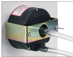
Mounting hardware is supplied with the Minihelic<sup>®</sup> II gage for panel mounting through a single hole, 2-5/8" (67 mm) in diameter. Panel thickness up to 1/2" (13 mm) can be accommodated with the hardware supplied. If necessary, surface mounting of the gage can be accomplished by means of two 4-40 screws into the tapped mounting bracket stud holes in the rear of the gage. Surface mounting requires clearance holes in the panel for the two pressure taps.
