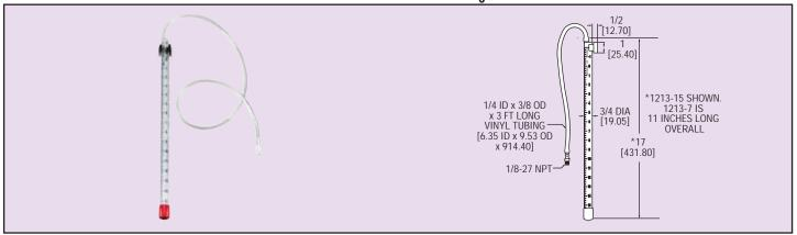
Provide visual indication of pressure with the Series 1213 Gas Pressure Manometer. Designed for use with natural gas, the manometer can also be used to monitor any compatible gases up to 15 inches of water column. Tap water is used as the sensing media and a magnetic clip provides temporary or permanent mounting. Economically priced and made of durable plastic for years of trouble-free service. Includes three feet of vinyl tubing and 1/8° nylon male NPT to barb fitting.
