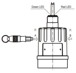
Make sure that after programming, the unit will not be exposed to a strong magnetic field!
