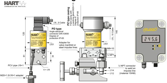
APRE-2000G Economic Version, process connection with terminal connecting to ∅6 pipe (PCV type) An example with PD type Electrical Connection
